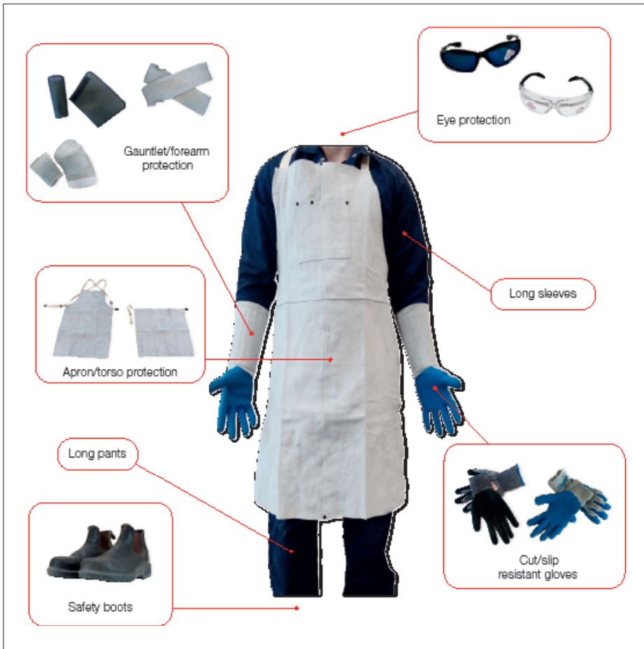
Figure 37 PPE for Glass Handling Source: Work Cover NSW
