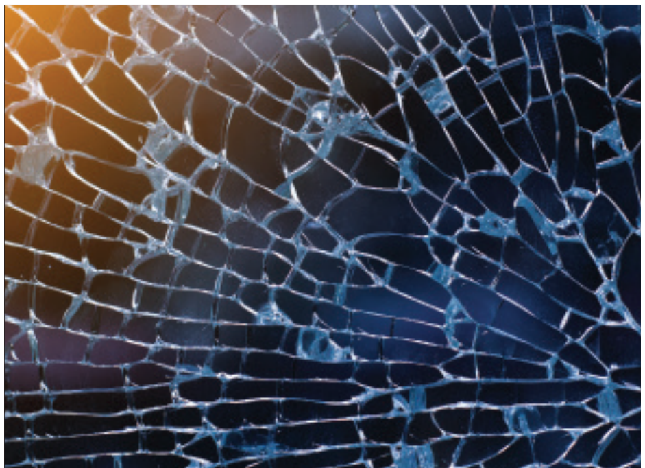
Figure 7 Toughened Glass When broken, toughened glass fractures into small granules. Source: Shutterstock
